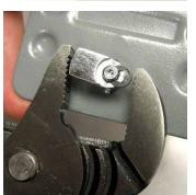
**Step 5**Snap the lock ring into position.
