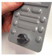
**Step 2**Rotate the Cam clockwise to the 'unlock' position.
